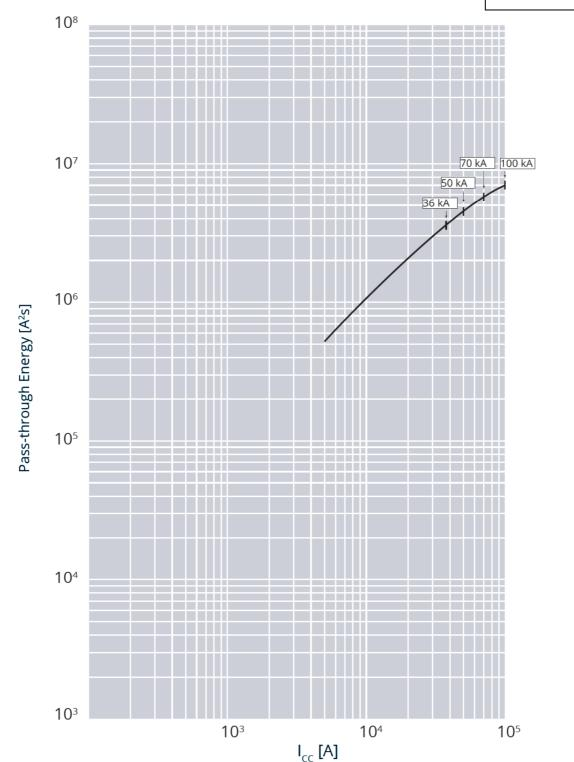
$I_{cu}$  = 36-50-70-100 kA  $I_{max}$  = 630A 3-4 P  $U_{e}$  = 415Vac (IEC/EN 60947-2)
