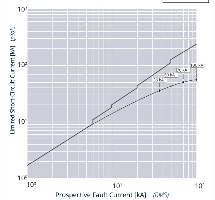
I<sub>ou</sub> = 36-50-70-100 kA I<sub>max</sub> = 630A 3-4 P U<sub>e</sub> = 415Vac (IEC/EN 60947-2)
