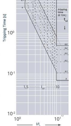
$I_{cu}$  = 36-50-70-100 kA  $I_{max}$  = 630A 3-4 P  $U_{e}$  = 415Vac (IEC/EN 60947-2)
