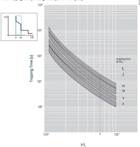
$I_{cu}$  = 36-50-70-100 kA  $I_{max}$  = 630A 3-4 P  $U_{e}$  = 415Vac (IEC/EN 60947-2)
