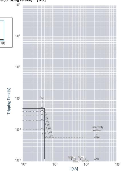
$I_{cu}$  = 36-50-70-100 kA  $I_{max}$  = 630A 3-4 P  $U_{e}$  = 415Vac (IEC/EN 60947-2) Fixed Instantaneous override  $I_{sf}$  = 5kA
