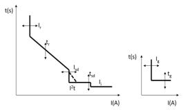
Long delay protection against overloads with an adjustable threshold bases on the RMS value of the current:
