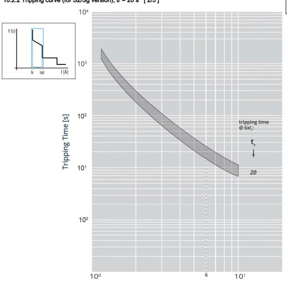
$I_{cu}$  = 36-50-70-100 kA  $I_{max}$  = 630A 3-4 P  $U_{e}$  = 415Vac (IEC/EN 60947-2)
