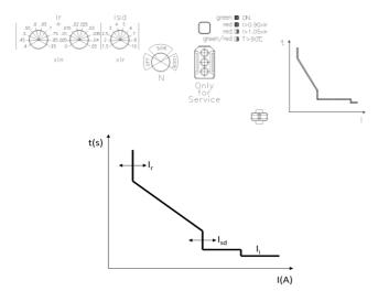
Long delay protection against overloads with an adjustable threshold bases on the RMS value of the current:
