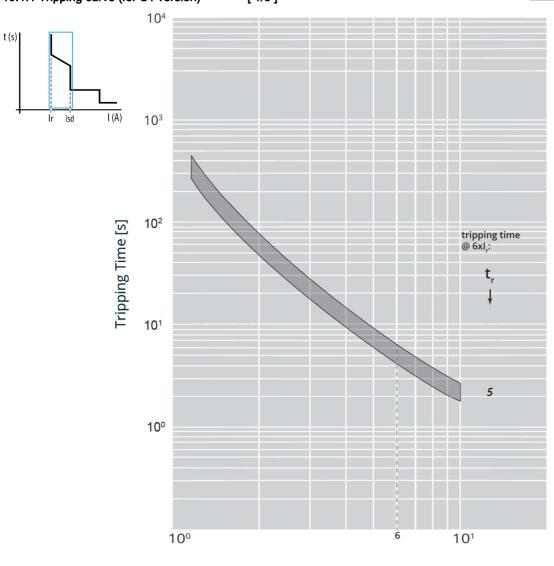
$I_{cu}$  = 36-50-70-100 kA  $I_{max}$  = 630A 3-4 P  $U_{e}$  = 415Vac (/EC/EN 60947-2)
