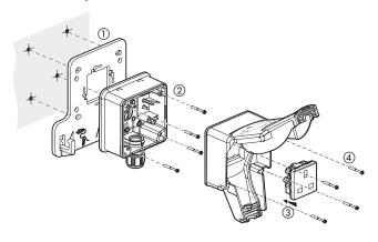
The front part (mechanism cover) is attached to the box using 4 coarse pitch screws.
