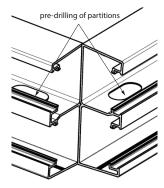
$\label{eq:constraints} \mbox{Double perforations of the bottom of the trunking for an easier levelling}$
