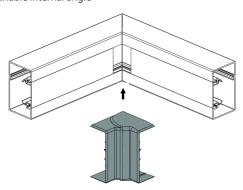
Enables the junction in internal angle of two pieces of the same section:
