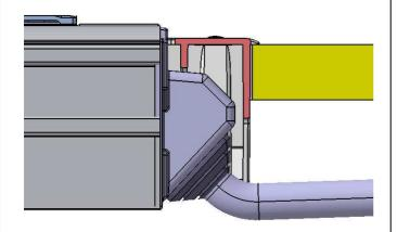
Section of the module with position of cable after end caps screwing and installation of cover plates.
