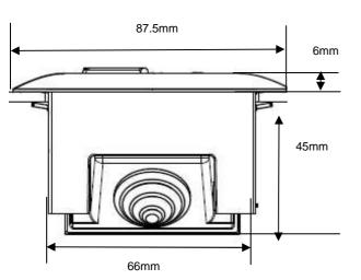
Minimum thickness to install in the wall :
