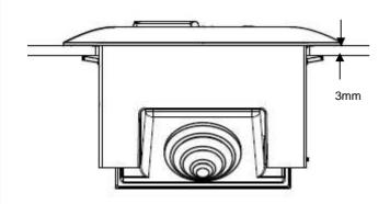
Maximum thickness to install in the wall :
