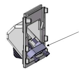
End cap with cable clamp integrated for an optimal safety
