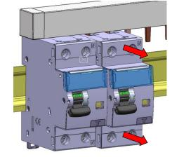
Pull the device downward in order to release it completely from the prongs of the busbar
