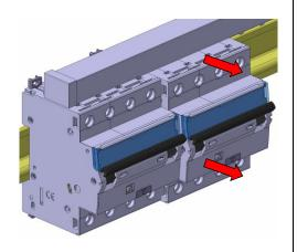
Pull the device downward in downward in order to release it completely from the prongs of the busbar
