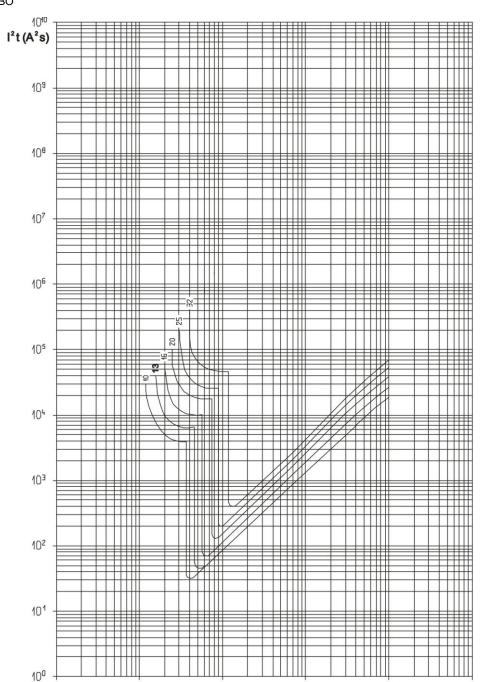
100  $\label{eq:lcc} \begin{array}{l} Icc = Prospective \ short-circuit \ symmetrical \ current \ (rms \ value \ in \ kA) \\ I^2t = Limited \ thermal \ stress \ (in \ A^2s) \end{array}$
