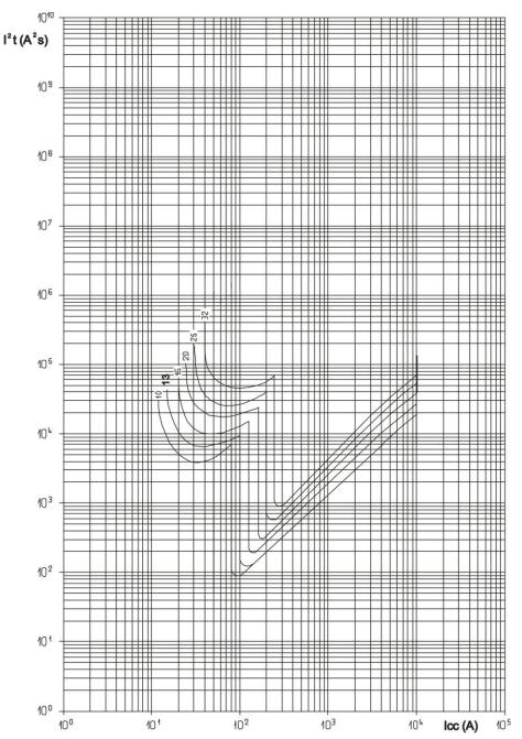
lcc = Prospective short-circuit symmetrical current (rms value in kA)  $I^2t$  = Limited thermal stress (in  $A^2s$ )
