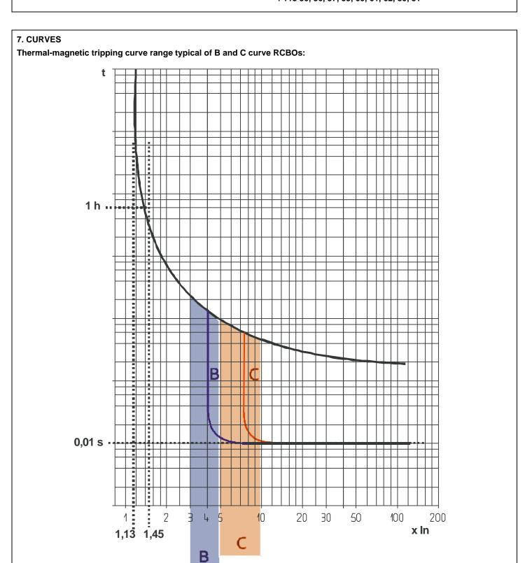
Thermal tripping at ambient temperature = 30°C In = RCBO rated current
