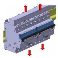
Put the clamp in the unlocking position
