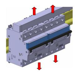
Put the clamp in the unlocking position
