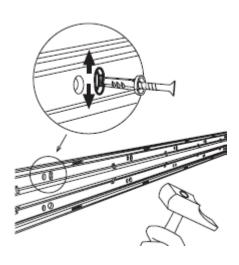
pipes can be pre-installed using pipe retainers positioned on the bottom as required, before being held in place by pipes ties.
