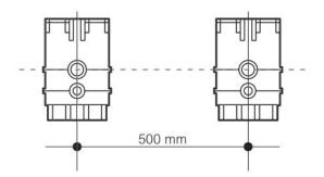
It is recommended that pipe clips are fitted every 50cm to ensure alignment
