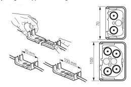
Place and hook the pipes with a pipe tie
