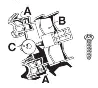
Adjusting the support according to the diameters (ranging from 10 to 22mm)
