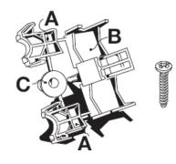
Adjusting the support according to the diameters (ranging from 10 to 22mm)
