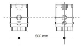
It is recommended that pipe clips are fitted every 50cm to ensure alignment
