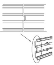
Oblong perforations in the bottom for quick fitting and easy adjustment of the base.
