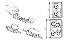
Place and hook the pipes with a pipe tie
