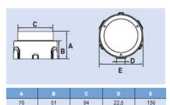
The plastic floor box fixes itself on the ground (with screws) using mounting feet
