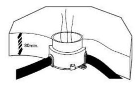
For information, in a use with concrete it is necessary to stop the hole of plastic floor boxes with adhesive tape or paperboard for example before put the concrete.
