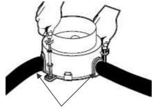
Possibility to put the plastic floor boxes with sheaths ICTA of  $\varnothing$  20 or 25mm
