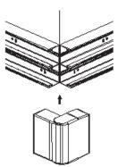
For information, on trunking 85x50, clip-on the adaptor (delivered with) on the two sides inside the angle:
