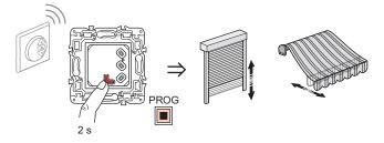
8.2.4 Removing a transmitter with an integrated inaccessible RTS receiver
