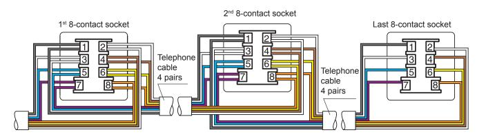
Wire sockets in parallel: all wires must be connected. Use France Telecom-approved 4-pair cable,  $\emptyset$  0.6 mm, type 278-4.6 Comply with the contact numbers and the wire colours.
