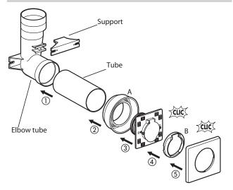
This installation outlet can be mounted on a peripheral wall, on a partition wall, or in a cupboard.
