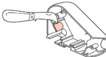
To fit a second cable, take out the part as shown above
