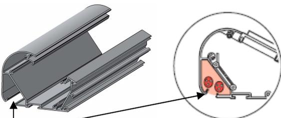
Enable you to fit 2 cables 3G 1.5 mm<sup>2</sup> or 3 data cables + 1 power cable.
