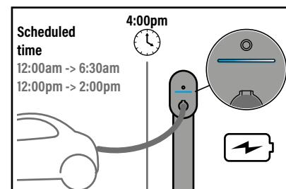
It is possible to start the charge at any time by overriding with a long press on the button on the front of the charging station or via the Home + Control app.
