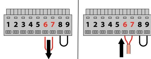
Remove the jumper from inputs 6 and 7 and connect the control device (e.g., time switch).
