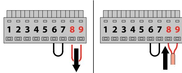
Remove the jumper from inputs 8 and 9 and connect the control device (e.g. time switch, contactor...).
