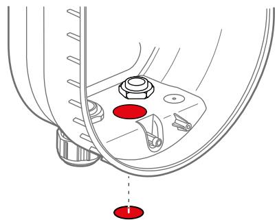
**💡 In the case of cable entry from the rear or for pedestal mounting** (see assembly steps in the instruction sheet), it is necessary to remove the cable glands fixed on the charging station and seal these entries with the cable glands (provided with the pedestal, or Cat.No 0 019 55, to be ordered separately). It is then necessary to drill the rear cable entries (non-knockout) with a step drill bit
