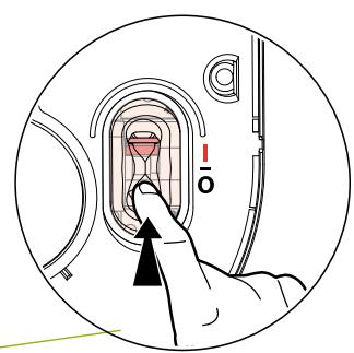
Flexible protection membrane to operate the RCBO lever
