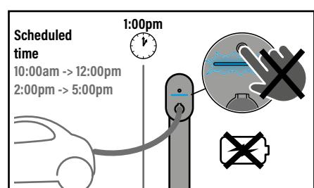
The override on the front button does not allow vehicle charging outside of the scheduled times.
