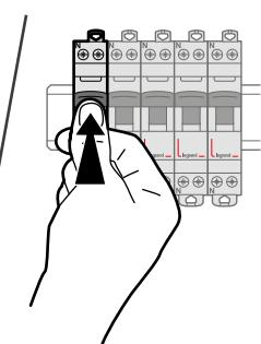
1. Power on the circuit in the panel and in the charging station (for version with built-in protection).
