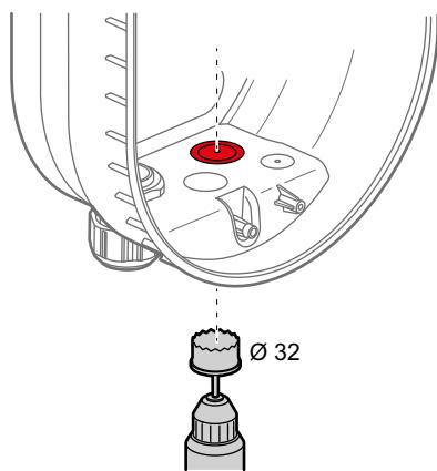
Use a membrane gland to seal an unused cable entry and ensure IP55 protection
