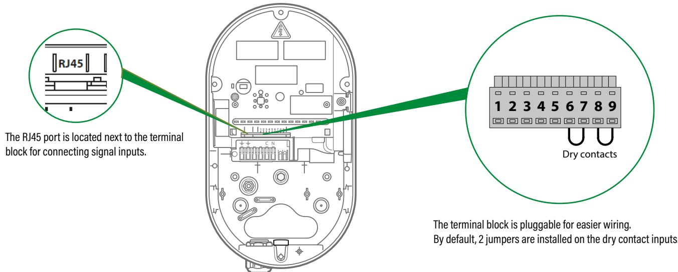
The RJ45 port is located next to the terminal block for connecting signal inputs.
