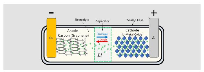
Figure 3: Li-Ion batteries chemical composition
