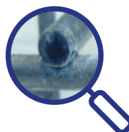
Blackening on the end of the wire
