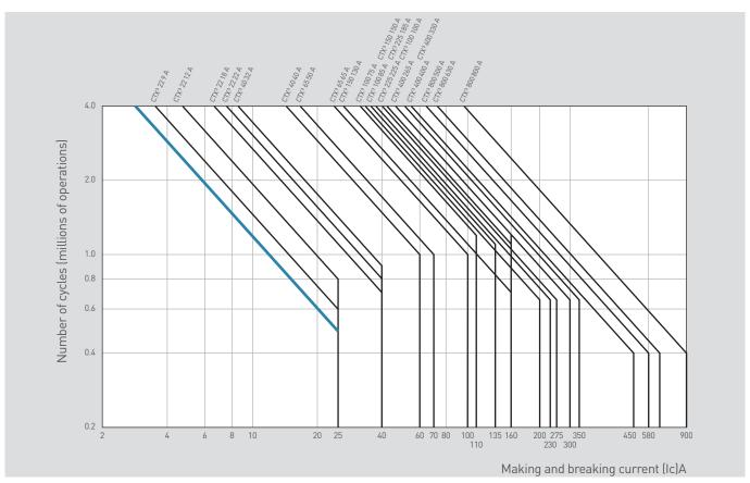
Example: For an AC-1 operating current of 50 A and endurance of 2 million operations for an external ambient temperature below  $40^{\circ}$ C, you should select a 65 A CTX<sup>3</sup>.
