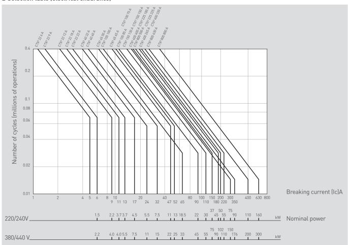
Example: Ic = 6 x Ie = 66 A for a 5.5 kW motor, Ue = 400 V Ie = 11 A. For endurance of 200,000 operations, you should select a 22 A contactor. PROTECTION AND CONTROL OF THREE-PHASE ASYNCHRONOUS MOTORS | TECHNICAL GUIDE | 49
