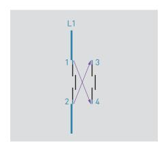
It is advisable to connect contacts in parallel by crossing over the connections, so as to divide the current equally in each
