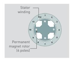
The rotor speed of rotation is characterised by the following equation:  $N = Ns = 120 \times (f)/No$ . of poles per phase.
