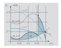
Sequence: when the speed of motor rotation stabilises (equilibrium between motor torque and resistive torque), at a speed of approximately 85% of nominal speed, the windings are then connected in a delta configuration and the motor regains its natural operating characteristics.
