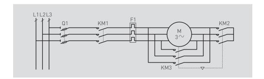
There is a method consisting of inserting a resistor before opening the star contactor to prevent the occurrence of transient phenomena associated with the sudden power cut. However, this process is rather more complicated and expensive to implement.
