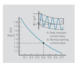
For a power factor on starting of 0.4, the inrush current reaches 1.3 times the normal starting peak current (7 x In x root of 2). If the motor restarts before the end of its rotation, this current surge can be twice as high. In this case, it can reach 2.6 times the nominal starting current, due to the residual current in the motor.
