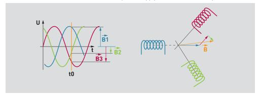
When supplied in this way, the stator generates a magnetic field, called a stator field, rotating at a speed called synchronous [Ns]. The rotation frequency of this field is linked to the frequency of the mains supply and the number of pairs of poles in the winding. Ns = 60xF/P (F frequency, P no. of poles), in number of revolutions per minute (RPM).
