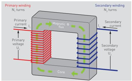
This magnetic field, channelled by a ferromagnetic core, passes through the secondary winding. Each turn in the secondary winding then creates a new induced voltage (back electromotive force).
