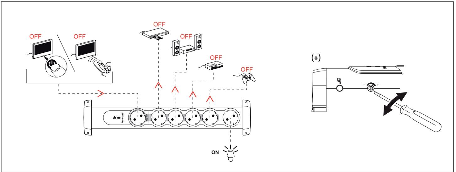
**GB** Connect your television or computer to the "MASTER" socket. When you turn off this device or put it on standby, power to the four controlled sockets is automatically cut off and any associated equipment plugged in to the unit is turned off.
