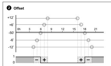
If the offset setting is in degrees the time switch switches on and off at times of equal brightness, despite the differences in twilight time lengths over the course of the year.
