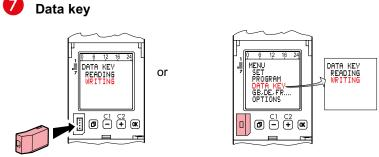
Load the programs of the time switch on to a data key (WRITE KEY) Warning! all programs stored on the data key will be overwritten.
