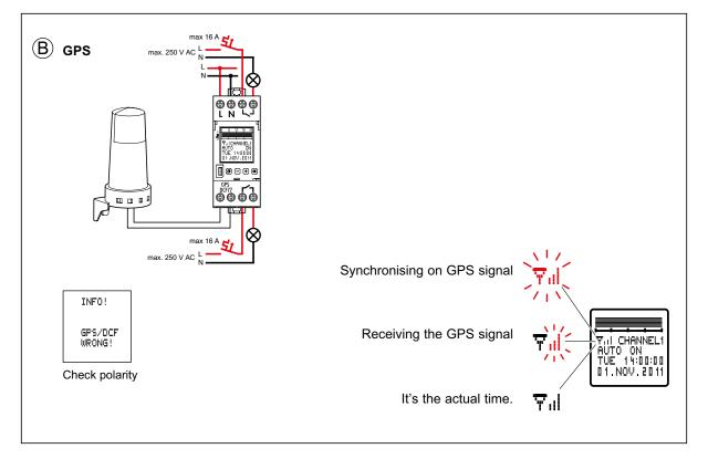
During normal operation the GPS-signal is actively decoded every 6 hours for 30 minutes. The time zone is not synchronised. A manual adjustment is necessary. By activating the expert mode the resolution of the coordinates can be increaded from degree to minute
