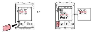
Load the programs from the data key to the time switch (READ KEY) Warning! all programs programmed in the time switch will be overwritten.
