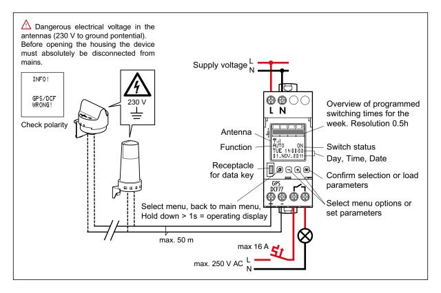
Antenna DCF77, reference 4 127 06 or antenna GPS, reference 4 127 07
