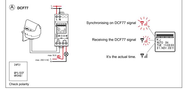
During normal operation, the DCF77 signal is actively decoded every 6 hour for 30 minutes.
