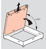
To remove the lid from the trim, hold it under an angle of approximately  $65^{\circ}$  and pull it out
