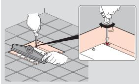
Make final adjustment to finished floor level by turning threaded rods in each corner with a screw driver
