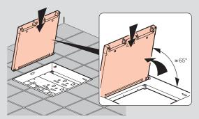
Push the lid back in place by holding it under an angle of approximately  $65^{\circ}$
