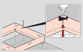
Make a rough adjustment to finished floor level by turning threaded rods in each corner with a screw driver
