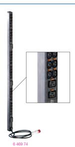
To provide  $\sim$  electric power for IT equipment in 19" enclosures Equipped with hydraulic magnetic circuit protection with high current interruption capacity. Hydraulic magnetic circuit breakers are not affected by ambient temperature 330° rotating cable input for a perfect orientation of the cable and no interference in the cabinet
