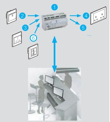
The Room Controller Unit, Cat.No 0 484 08 or 0 484 12, associated with mechanical Belanko™ S functions can manage the lights, sockets outlet, ventilation and curtains independently in each room. It can be integrated with the Building Management System (BMS) and the Property Management System (PMS) in order to enable a global management of the building and the hotel's operations.
