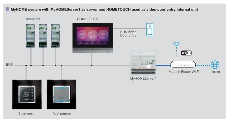
If MyHOMEServer1 is used to realize the MyHOME installation, the HOMETOUCH can be used as smart home touch screen and also as video door entry internal unit. Remote management of door entry function via the Door Entry App. for HOMETOUCH
