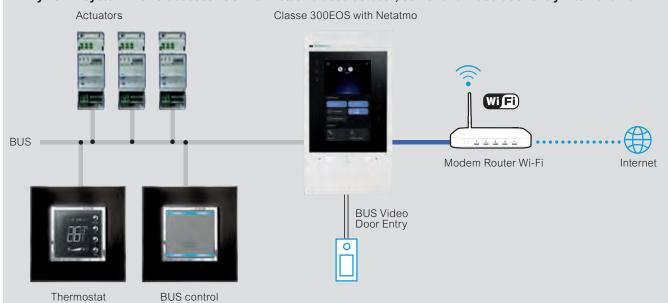
If Classe300EOS with Netatmo is used to realize the MyHOME installation, the device will work as both, smart home touch screen and video door entry internal unit. Remote management of door entry function via the Home + Security App.
