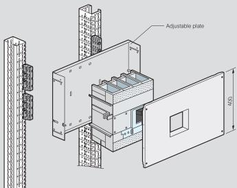
XL<sup>3</sup> 4000 - equipment for mounting on adjustable plates: DPX<sup>3</sup> 1600 draw-out version and supply invertors
