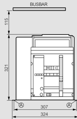
A = fixing point on plate of enclosure
