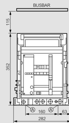
A = fixing point on plate of enclosure
