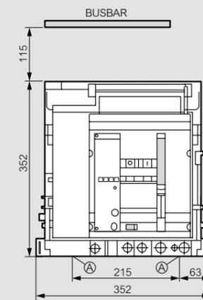
Rear terminals for horizontal connection with bars
