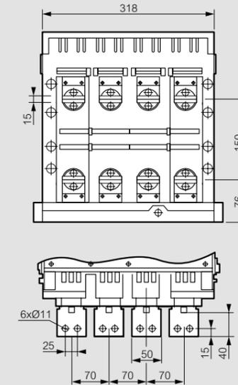
Rear terminals for vertical connection with bars
