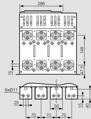
Rear terminals for vertical connection with bars
