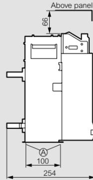
A = fixing point on plate of enclosure
