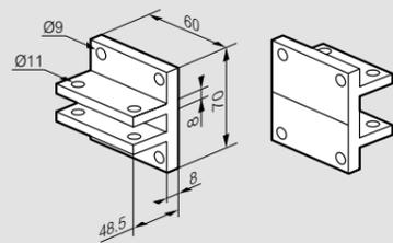
Rear terminals for vertical connection with bars
