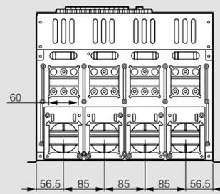
Rear terminals for horizontal connection with bars
