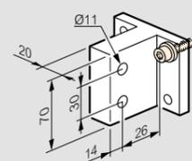
Rear terminals for vertical connection with bars
