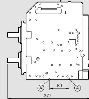
A = fixing point on plate of enclosure
