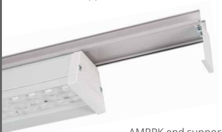
AMRPK end support and lower bracket which can be fastened by screw or by pressing together must be ordered separately. With the lower bracket the ramp luminaires installed between the lighting suspension rails can be positioned on the same level as luminaires installed to the lighting suspension rail with AMJK2 spring brackets.
