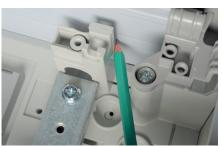
Use the terminal block supports as marking
