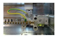
XL<sup>3</sup> 160 enclosures are supplied with a brass bar for protective conductors with  $2 \times 35 \text{ mm}^2$  holes and  $36 \times 10 \text{ mm}^2$  holes. As the cabinet is reversible, the bar can be placed at the top or the bottom.
