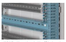
XL $^3$  160 cabinets also take Lina 25 horizontal ducting: use insulating screws Cat. No. 0 367 74 [M6x10 mm screws) to fix them horizontally (40 x 60) directly on the uprights.
