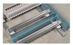
XL $^3$  160 cabinets also take Lina 25 horizontal ducting (40 x 60): use insulating M6x10 mm screws Cat. No. 0 367 74 to fix the ducting directly on the uprights
