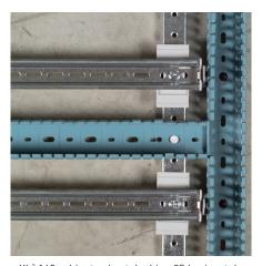
XL<sup>3</sup> 160 cabinets also take Lina 25 horizontal ducting: use M6x10 mm insulating screws Cat. No. 0 367 74 to fix the ducting directly on the uprights
