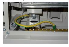
$XL^3$  160 cabinets are supplied with a brass terminal block for protective conductors with 2 x 35 mm<sup>2</sup> holes and 36 x 10 mm<sup>2</sup> holes. As the cabinet is reversible, the terminal block can be placed at the top or the bottom.
