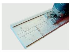
The side panels are easy to cut using a jigsaw
