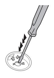
Knock out the holes corresponding to the position of the lugs  $% \left\{ \left( 1\right) \right\} =\left\{ \left($
