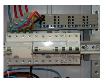
$\bullet$  Three-phase vertical distribution using auto VX³ supply busbar available in 63 A (3, 4, 5 and 6 rows) or 125 A (4, 5 and 6 rows). These models are equipped with automatic output terminals.
