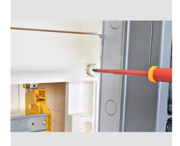
We recommend using a 6.5 mm flat screwdriver to open and close the  $XL^3$  125 cabinets, and also for positioning the faceplates with a  $\frac{1}{4}$  turn, for which 1 nm tightening torque is sufficient.
