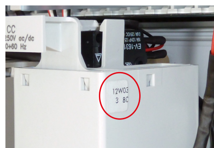
For all accessories, the date of manufacture is marked on a small sticker, as well as on the packaging label.
