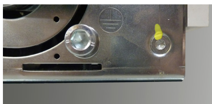
Connection point on the fixed DMX 3
