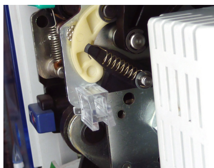
Accessory for correct adjustment of the supply inverter connecting rod
