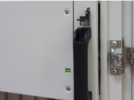
The tray position is indicated by a coloured LED and can be locked out with a padlock.
