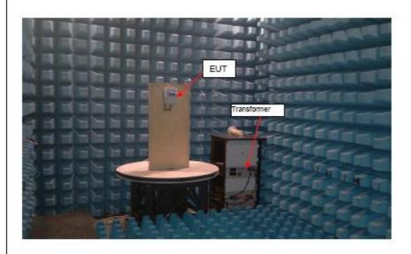
Note: Distance from EUT to aerial: 3 m Height of the EUT from the ground: 1,5 m
