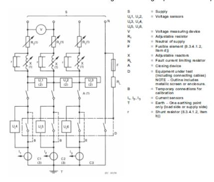
Test circuit for the verification of short-circuit making and breaking capacities on three pole equipment
