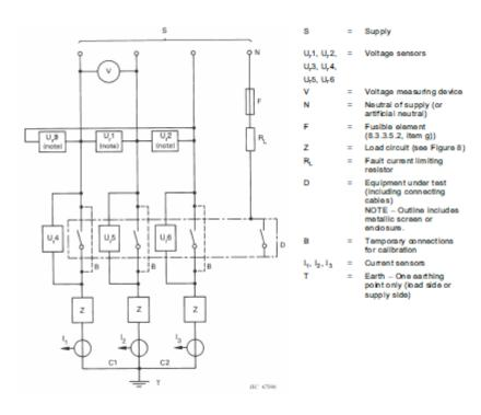
Test circuit for the verification of making and breaking capacities on three-pole equipment
