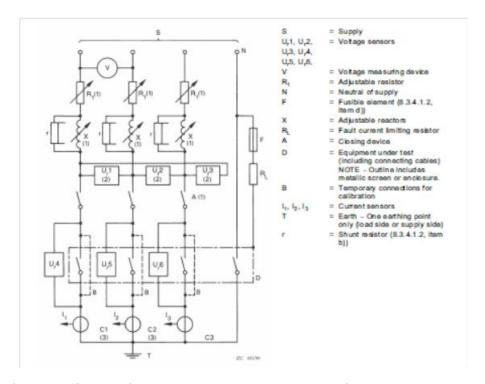
Test circuit for the verification of making and breaking capacities on four-pole equipment Three fase test carried out on N-L1-L2
