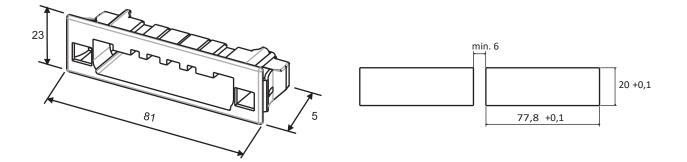
The dimensions of the mounting hole of the panel mounting adapters are shown in the figure. Make sure that the dimensions are accurate after the plate has been painted. Plate thickness 0.5 – 1.5 mm.
