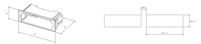
The dimensions of the mounting hole of the panel mounting adapters are shown in the figure. Make sure that the dimensions are accurate after the plate has been painted. Plate thickness 0.5 - 1.5 mm.
