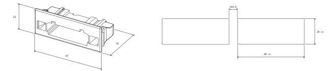
The dimensions of the mounting hole of the panel mounting adapters are shown in the figure. Make sure that the dimensions are accurate after the plate has been painted. Plate thickness 0.5 – 1.5 mm.
