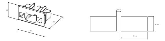
The dimensions of the mounting hole of the panel mounting adapters are shown in the figure. Make sure that the dimensions are accurate after the plate has been painted. Plate thickness 0.5 - 1.5 mm.
