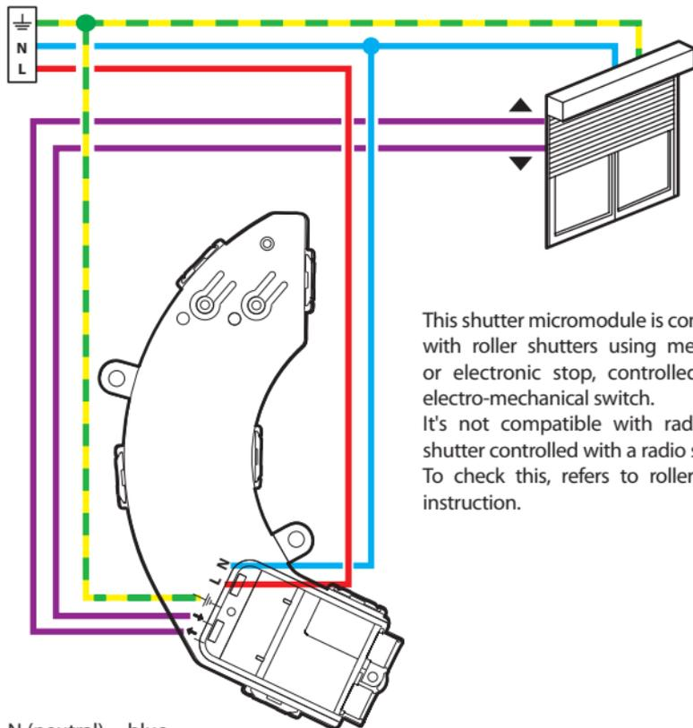
This shutter micromodule is compatible with roller shutters using mechanical or electronic stop, controlled by an electro-mechanical switch. It's not compatible with radio roller shutter controlled with a radio switch. To check this, refers to roller shutter instruction.
