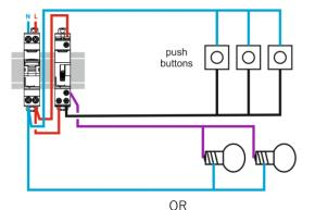
Installation « 4 wires » with line on the push-buttons
