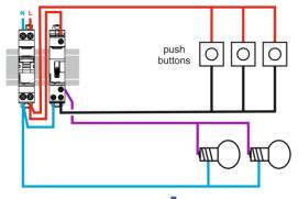
After: Installation « 4 wires » with line on the push-buttons
