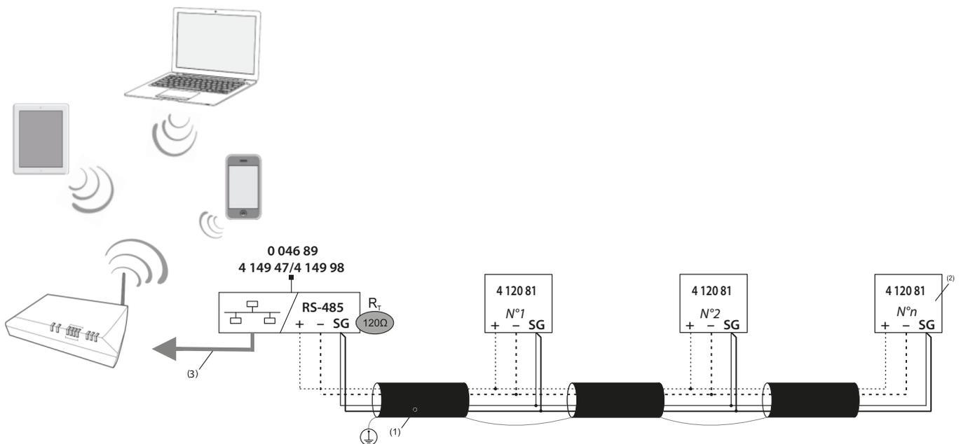
(1) RS485: Required use of Belden 9842 or Belden 3106A wire (or equivalent) for a maximum bus length of 1000 m, or Category 6 wire (FTP or UTP) for a maximum length of 50 m
