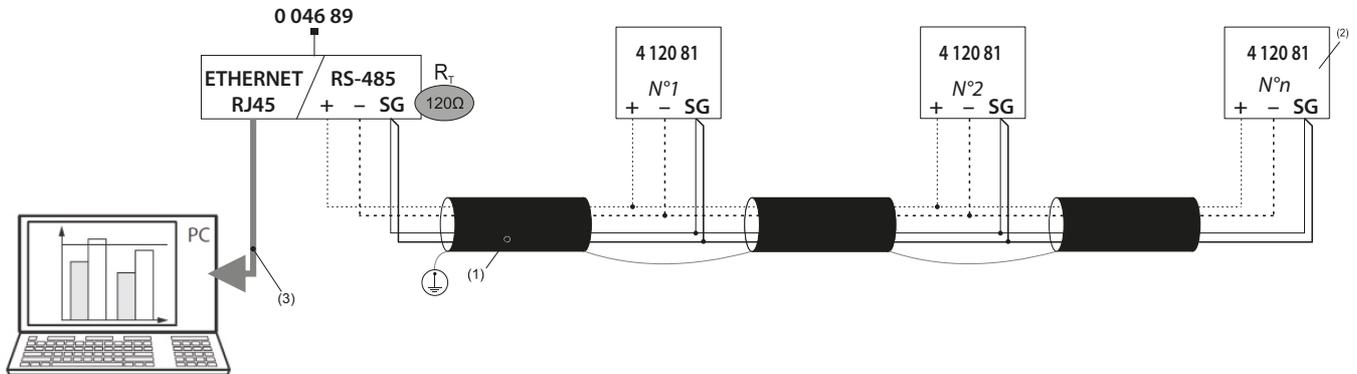
RS485 Modbus wiring diagram with Mini Web Server:
