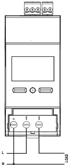
Terminal board marking and diagram combination:
