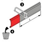
. Cut the protection plastic cover to the required length
