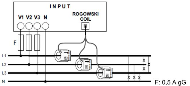
4 wires three-phase network, 3 sensors (3N-3E):
