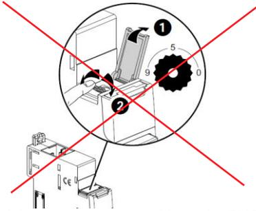
. It is not necessary to address the EMS CX<sup>3</sup> modules. The track wheel must be left in default position "0".
