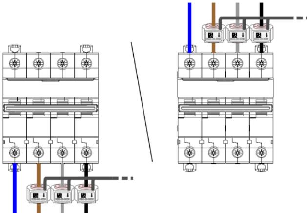
. Rogowski coils must be put in the correct direction of current flow (**arrow drawing on the coil**).
