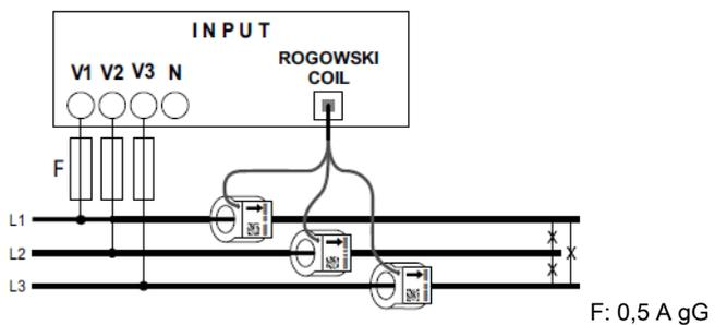
. Rogowski coil(s) cable length (see § Overall Dimensions) allow you to put EMS CX<sup>3</sup> Measure modules everywhere in the installation. This is not mandatory to have them near to the associated protection device of the measured line.
