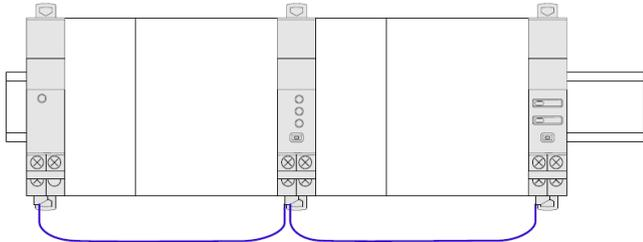
**Implementing:** with this configuration, the plastic protection cover of the backside communication ports on the EMS CX<sup>3</sup> module must be kept on.
