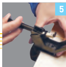
Align the fibre
