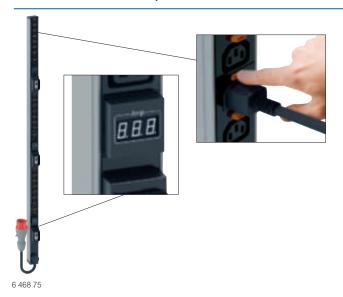
To provide ~ electric power for IT equipment in 19" enclosures Three phase Zero-U PDUs for vertical mounting in the cabinet 380 V - 50/60 Hz power supply Each circuit is protected by 16 A single pole MCB in a support with projecting edges to avoid accidental breakdown. 1 circuit per phase, each with 6 IEC 60320 C13 outlets and 2 IEC 60320 C19 outlets 230° extrapolations. 330° rotating cable input for a perfect orientation of the cable and no interference in the cabinet
