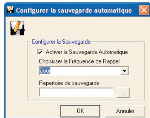
You can configure an automatic backup. In this case, the user is reminded that an installation backup must be performed at scheduled intervals: daily, weekly or monthly.
